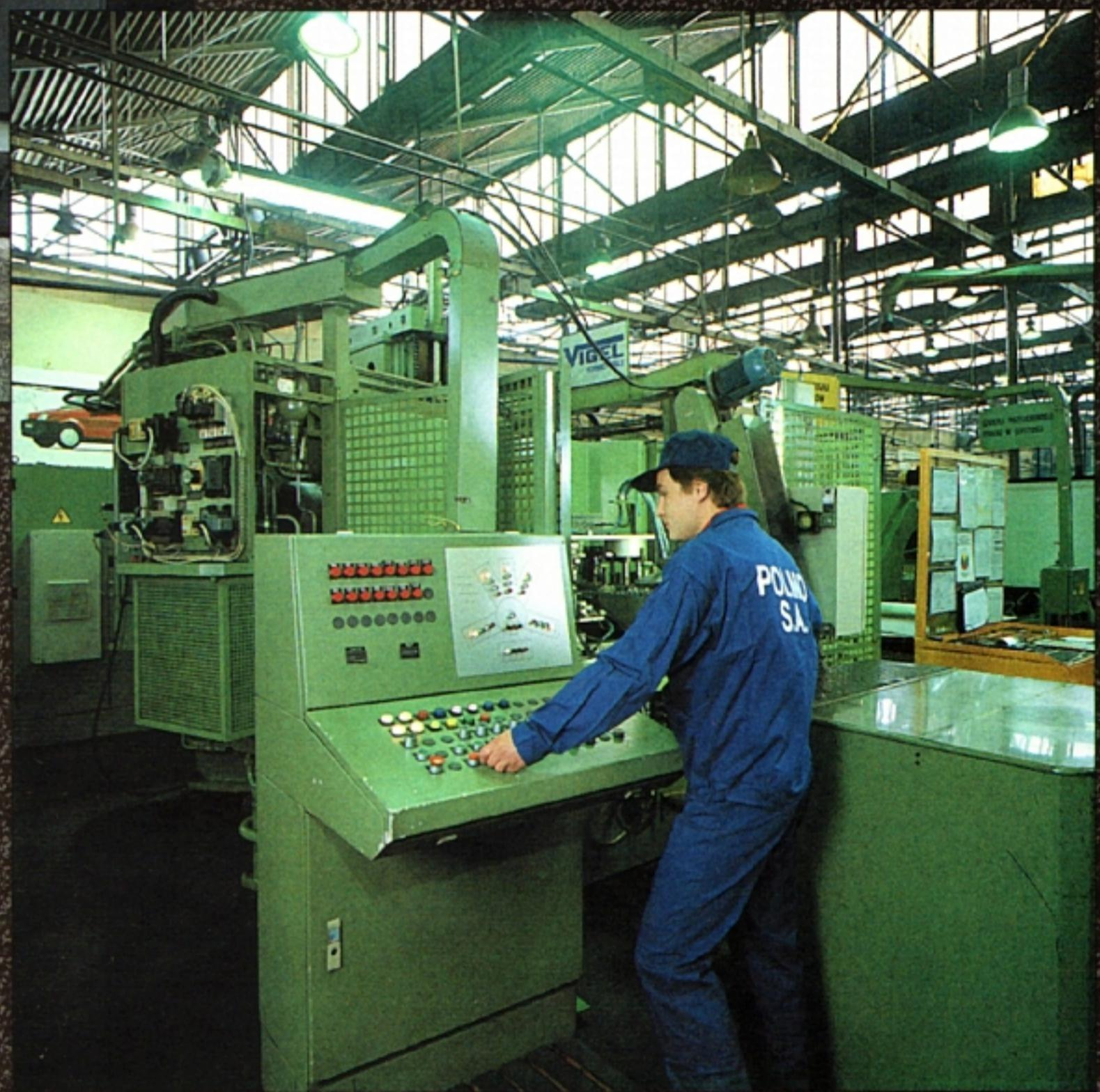
In 1964 drive shaft production was started, which initiated the later taken course of activities in the company. In 1967 the company has taken the name of Factory Of Car Mechanisms "POLMO" Co. During the last decades the factory has stabilized its production profile. It started to specialize in production of steering shafts, drive shafts and steering gears for all types of automobiles made in the country.
